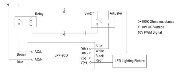
Using a switch and relay can turn ON/OFF the lighting fixture.
