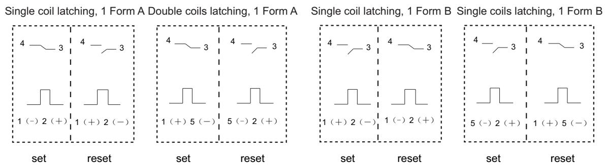
**Wiring Diagram (Bottom view)****HFE20-1
