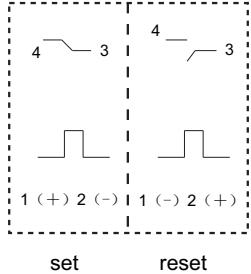
Single coil latching, 1 Form B Double coils latching, 1 Form B
