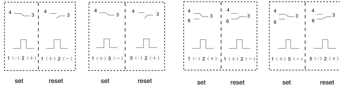
Single coil latching, 1 Form B Double coils latching, 1 Form B
