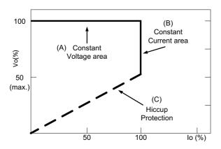
Typical LED power supply I-V curve
