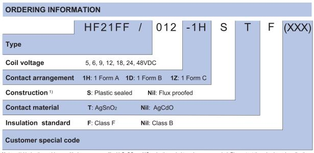
Notes: 1) Under the ambience with dangerous gas like H<sub>2</sub>S, SO<sub>2</sub> or NO<sub>2</sub>, plastic sealed type is recommended; Please test the relay in real applications. If the ambience allows, flux proofed type is preferentially recommended.
