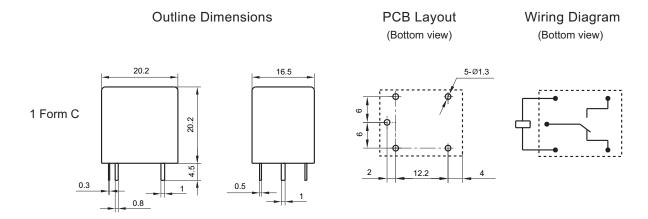
Remark: 1) In case of no tolerance shown in outline dimension: outline dimension  $\leq$ 1mm, tolerance should be  $\pm$ 0.2mm; outline dimension >1mm and  $\leq$ 5mm, tolerance should be  $\pm$ 0.3mm; outline dimension >5mm, tolerance should be  $\pm$ 0.4mm.
